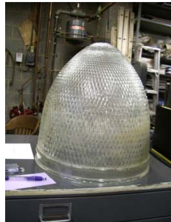
Figure 6 Teardrop shaped glass from cast iron cage fixture, at Charles Heim residence
